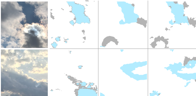
Fig. 6. Detailed comparison of cloud segmentation results - from left to right: input, Dev et al. [47], SkyCloudNet , ground truth
